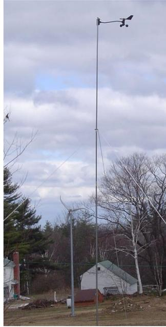
Figure 5-3: Sample image of a currently available wind measurement system mounted atop a dedicated pole, image source reference [30]
