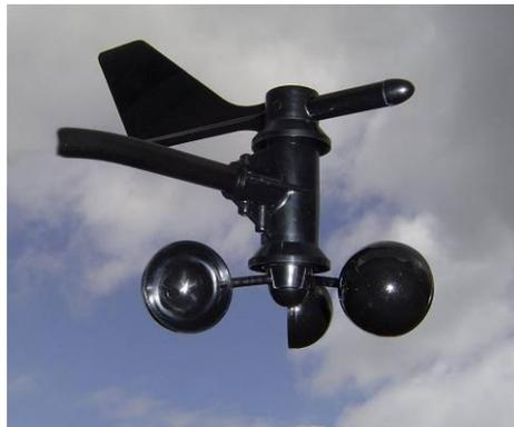
Figure 5-4: Close-up view of wind speed anemometer and wind direction sensor, image source reference [30]
