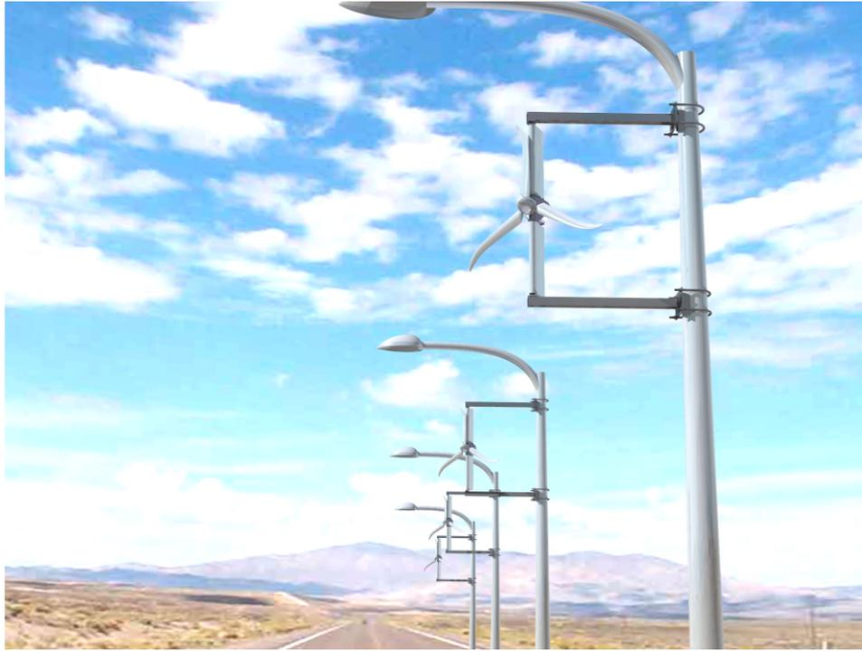
Figure 11-2: CATIA V5 render of sample installation on street light poles
