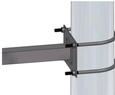
Figure 11-1: A U-bolt is used to attach the small wind turbine system to an existing pole
